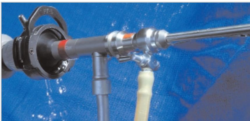
Figure 1 – Escaping fluid collects in the camera junction causing condensation and fogging.
